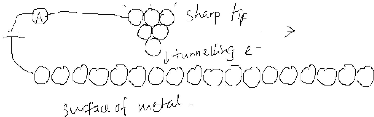
When a sharp tip is moved over a surface, tunnelling current changes with its spacing from surface atoms.
